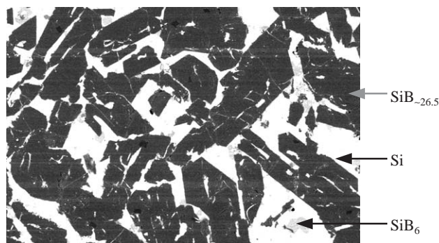
Fig. 1. Backscattered electron image of the sample with initial atomic composition B/Si=90/10. The phase \text{SiB}_n corresponds to large and elongated grains (black), while the binary \text{SiB}_6 is present as very small grains (gray). \text{SiB}_6 results from the peritectic reaction between \text{SiB}_n - and Si-rich liquid (white).
